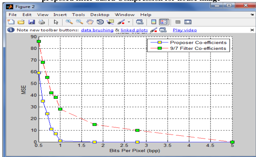
Figure-5 Comparison in MSE with respect to bpp for Wavelet 9/7 filter based compression and proposed filter based Compression for house image
