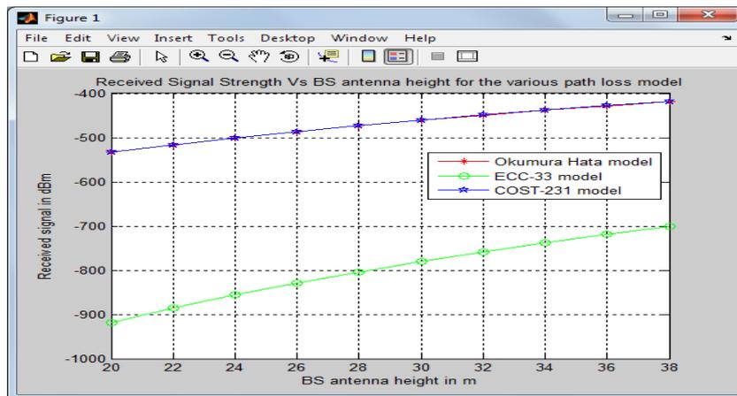
Figure 3: Plot showing received signal strength against BS antenna height for the various empirical propagation models
