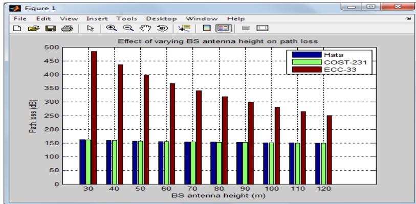
Figure 2: Bar chart showing path loss against BSAntenna height for the various empirical Propagation models
