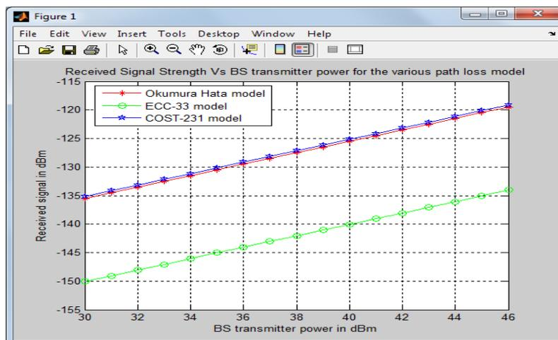
Figure 5: Coverage Prediction Plot showing the impact of transmitted power on coverage area (received signal strength)
