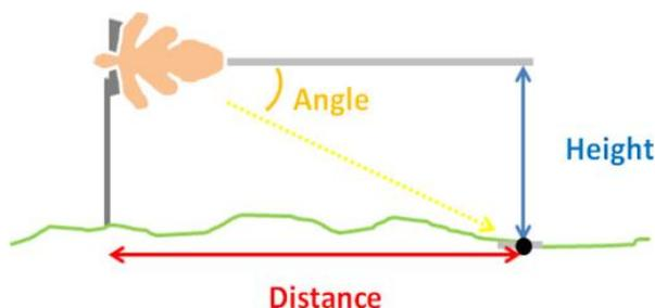
Figure1(c): Relationship between antenna height, tilt and T-R distance
