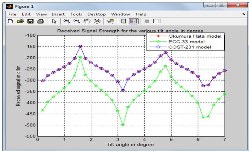
Figure 4: Plot showing the effect of tilt on Received signal level
