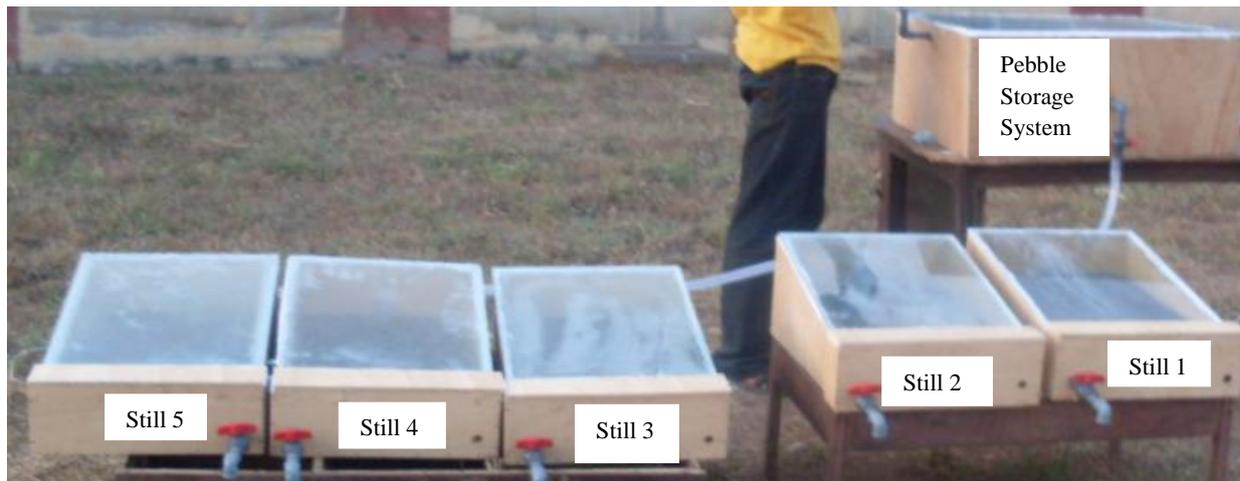
Plate 1: The set up of the five solar stills for the study
