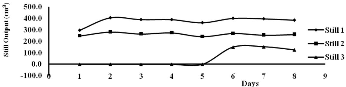
Fig. 3: daily still outputs for the 3 stills that distilled water
