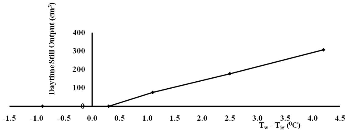
Fig. 2: variation of daytime still output with difference in temperature between the water and the inner glass surface
