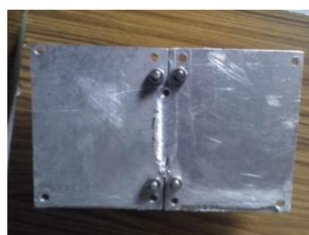
**Fig 4 (d)** specimens after FSW
