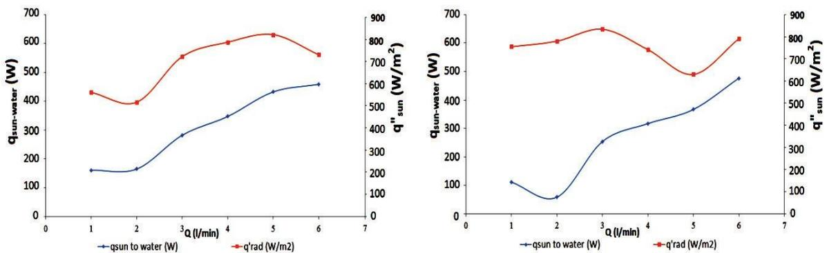
FIGURE 9. Data for serial (left) and parallel (right) pipe arrangements, CPC with glass cover
