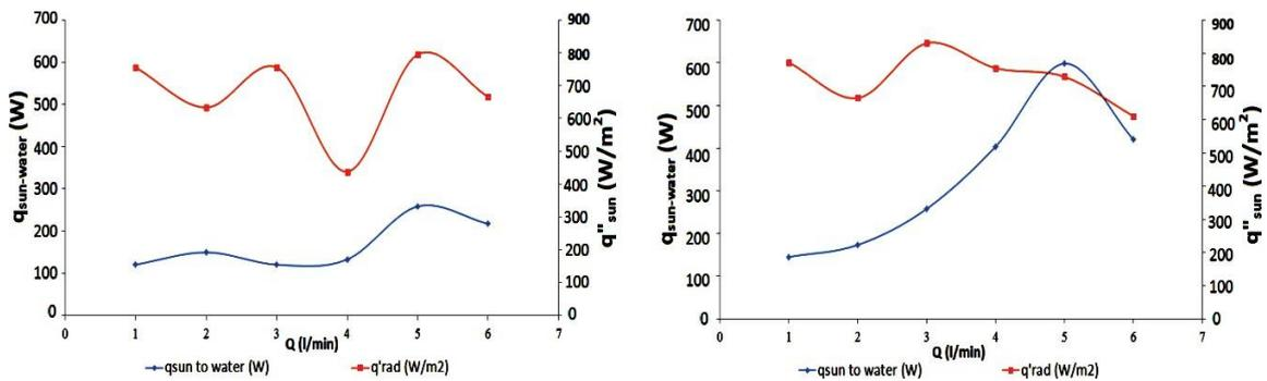
FIGURE 8. Data for serial (left) and parallel (right) pipe arrangements, CPC without glass cover
