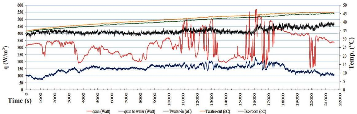
FIGURE 5. Data for 3 l/min flow rate, serial type flow, CPC without glass cover
