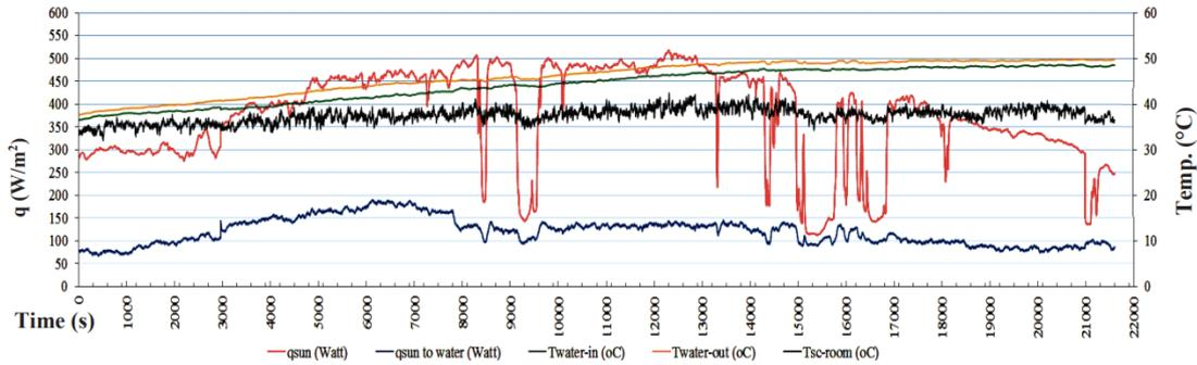
FIGURE 3. Data for 1 l/min flow rate, serial type flow, CPC without glass cover
