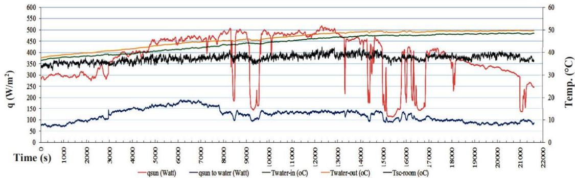
FIGURE 6. Data for 4 l/min flow rate, serial type flow, CPC without glass cover
