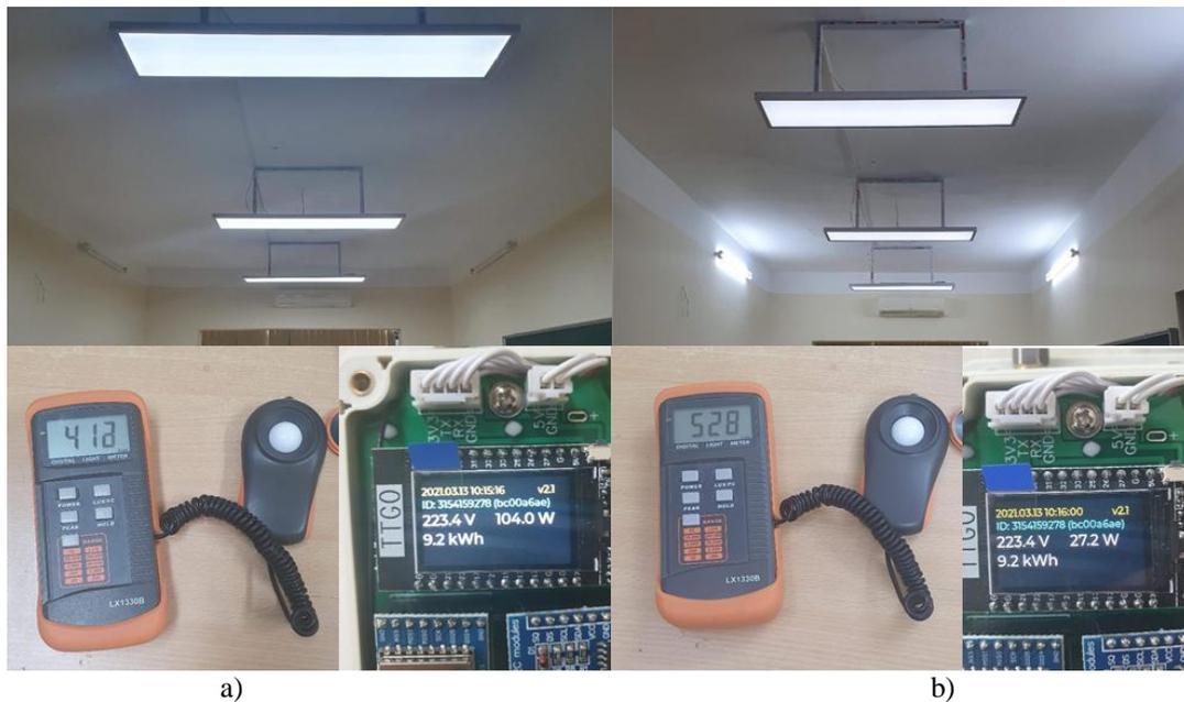
a) External light is ON: power consumption is 104W, illuminance is 418 lux; b) External light is OFF: power consumption is 27W, illuminance is 528W
