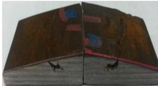
(a) Alloy steel ingot(b) Specimens shape
