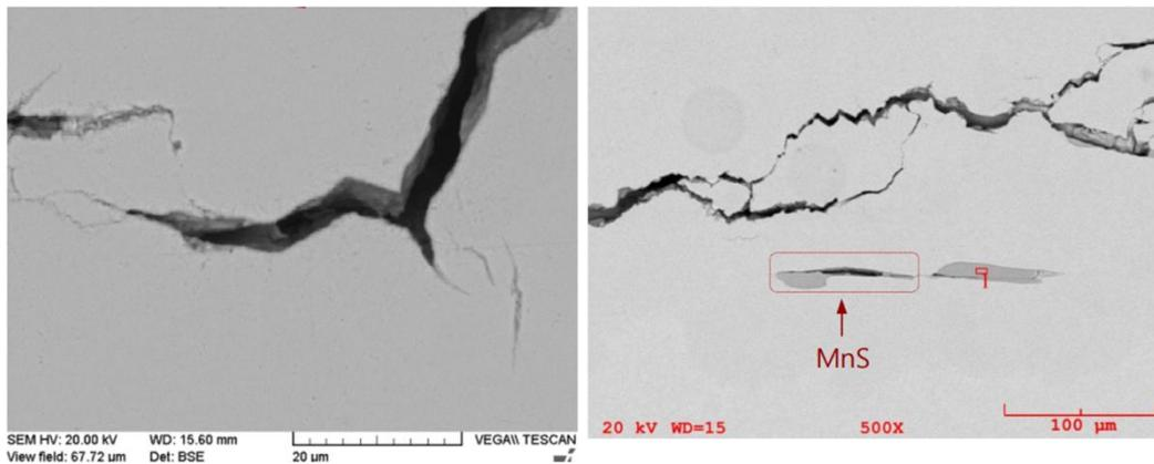
(a) Crack zone (500×) (b) MnS voids morphology of the crack zone (500×)
