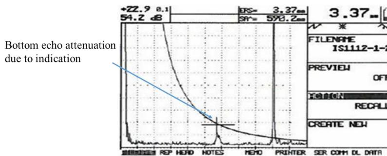
Indication size:  $\varnothing$  3.37 mm , Indication depth: 590.2 mm
