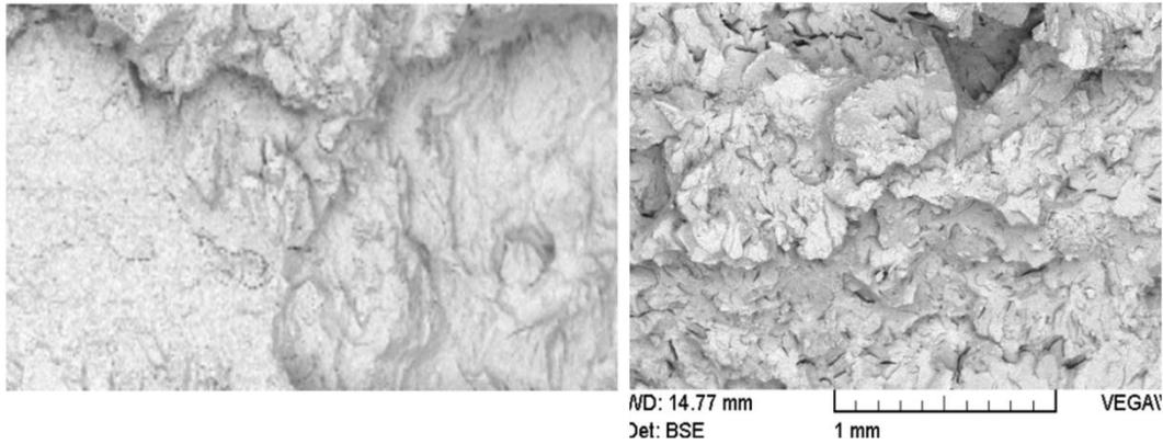
(a) forged crack surface (b) forced fracture surface
