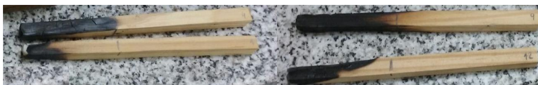
Figure 6. Untreated (up) and treated wood (down) after RIB test
