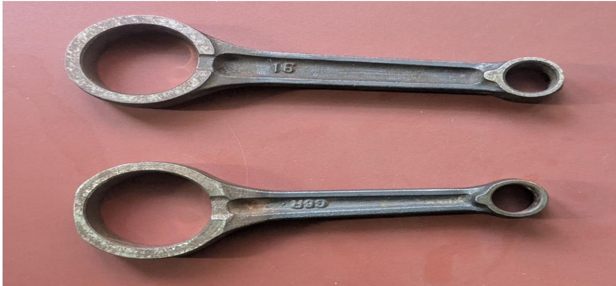
Fig-5: Actual connecting Rod made with carbon steel of BAJAJ PULSAR
