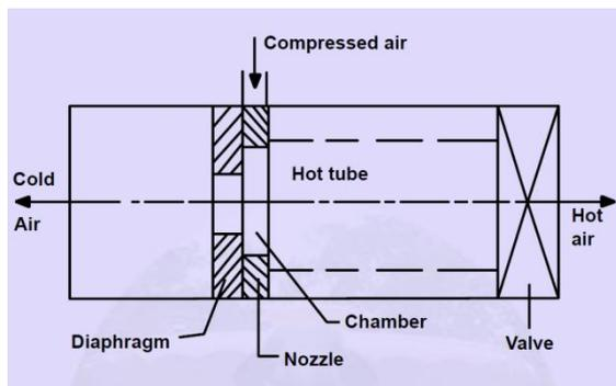
Figure 1.1: Schematic diagram of Vortex tube
