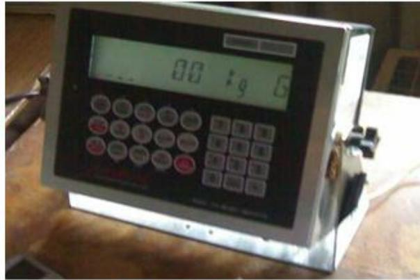
Plate 2: Axle weighing meter
