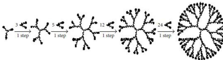
Figure 3: Stepwise synthesis of Dendrimers
