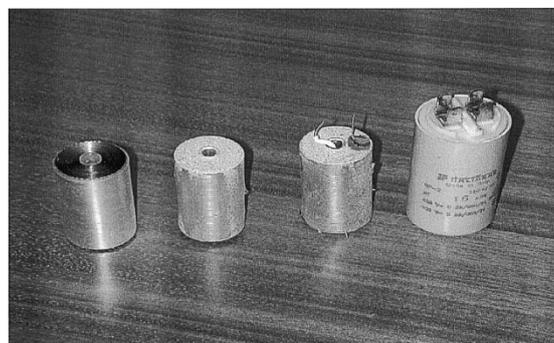
Fig.1: From left: the coiled cylindrical element: the element with the sprayed ends; the element with the two connection wires; and the complete capacitor.
