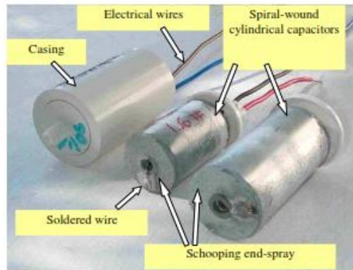
Fig. 2: Typical cylindrical low power MKP capacitors. The two removed from their cases are degraded through use.
