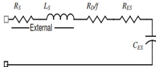
Fig.3: Modified capacitor equivalent circuit.
