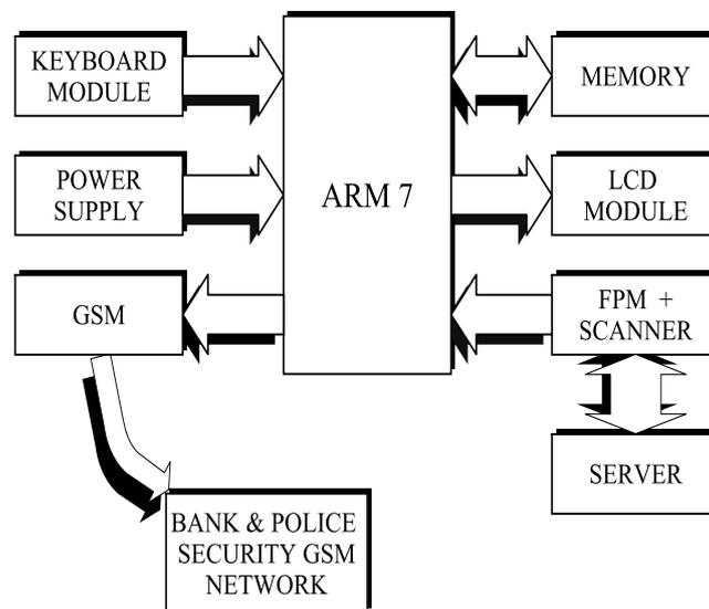
Figure 1: Basic block diagram of ATM security system
