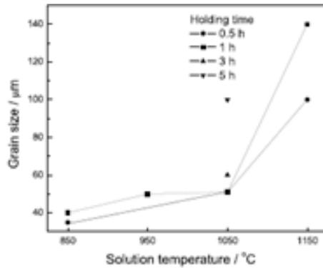
Fig. 11: Effect of solution treatment (ST) and holding time on PAG size on tested steel.
