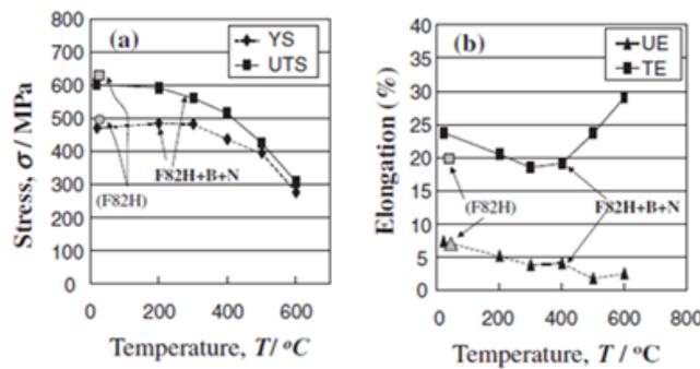
Fig. 8, 9: Tensile properties of F82H+60ppm+200ppm N steel
