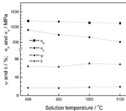
Fig. 12: Effect of ST temperature on tensile properties of tested steel in ST condition.
