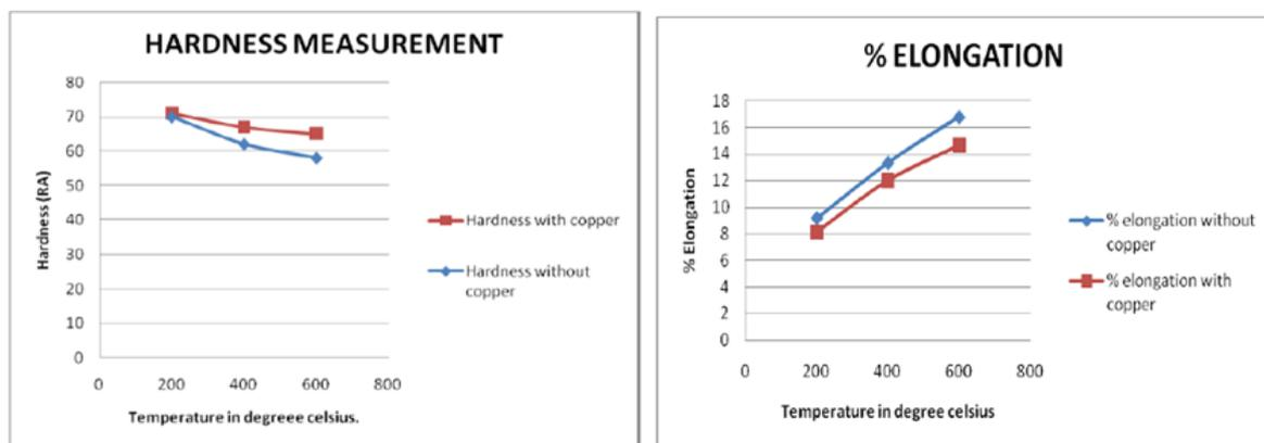
Fig. 7: Hardness and Elongation measurement
