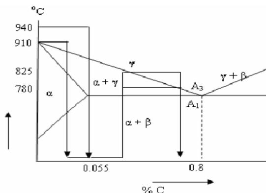
Fig. 5: Schematic heat treatment diagram: As received and intermediate quenching process  $\alpha$  Ferrite,  $\beta$ : Cementite,  $\gamma$ : Austenite
