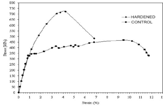
Fig.4: Stress and strain curve for hardned and control specimen
