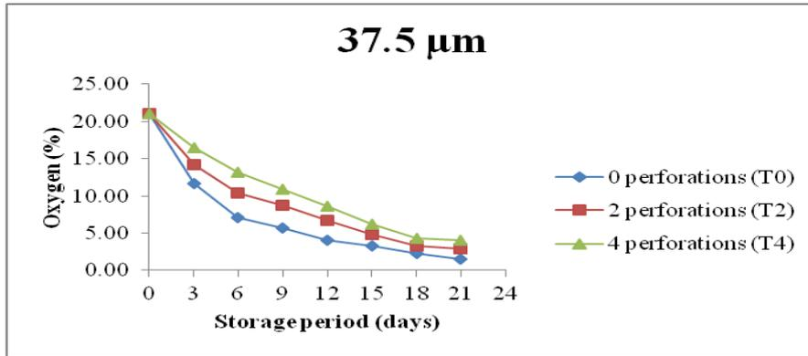
Figure 1: Oxygen concentration (%) for 37.5 μm thickness LDPE film at low temperature storage conditions
