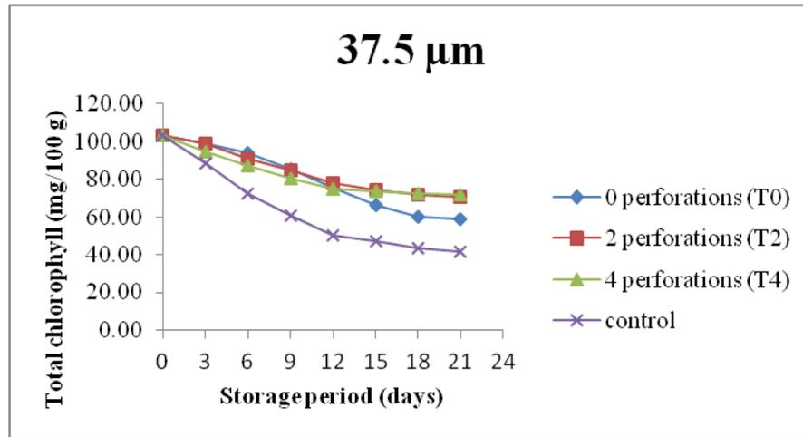
Figure 7: Total chlorophyll content (mg/100 g) for 37.5 µm thickness LDPE film at low temperature storage conditions
