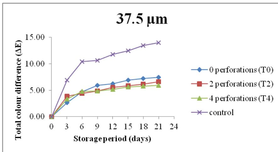
Figure 5: 'ΔE' values for 37.5 μm thickness LDPE film at low temperature storage conditions
