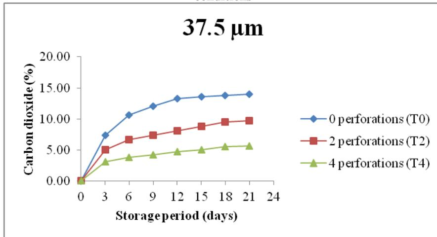
Figure 2: Carbon dioxide concentration (%) for 37.5 μm thickness LDPE film at low temperature storage conditions
