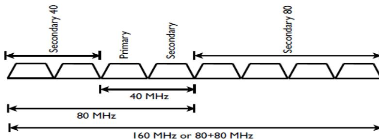
**Figure 2. Primary and Secondary channel selection**
