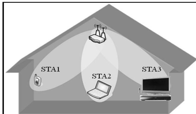
**Figure 3. Example of Downlink Multi User MIMO Network.**
