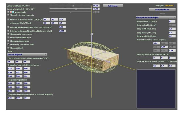
Figure 2. The inertia ellipsoid of the non-displaced moment of inertia tensor
