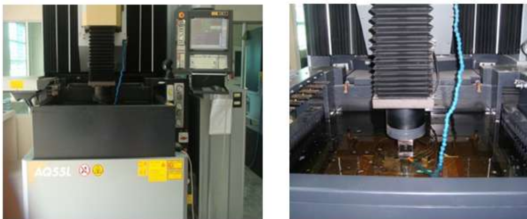
(a) Photograph of EDM during machining (b) EDM tank and sample at operational condition.
