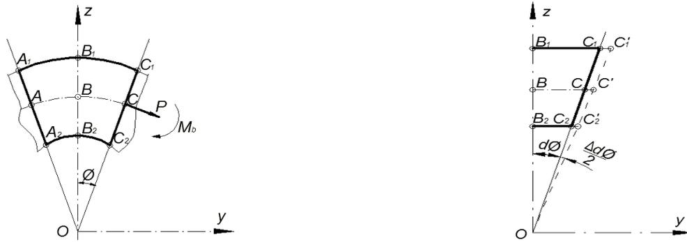
Figure 3 - Section of undeformed link (left) and section of deformed link (right)
