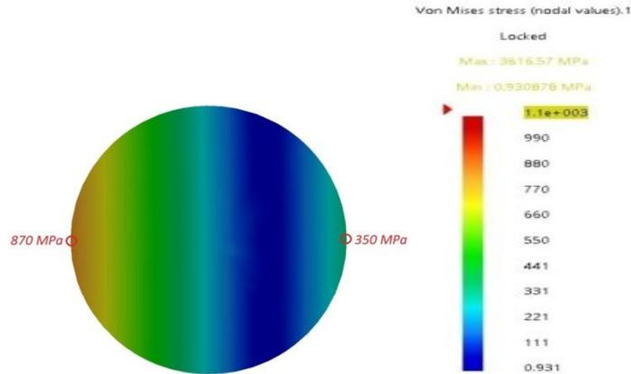
Figure 9 - The value of Von Mises stress in the middle of the link loaded with 80 kN
