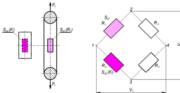
Figure 13 - Connection in 1/4 bridge with compensational measuring tapem
