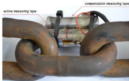
Figure 10 - Place with the active and compensational measuring tape
