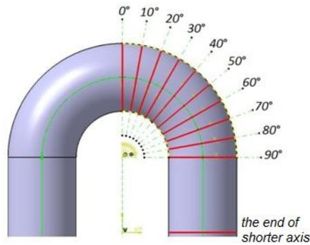
Figure 4 - Layout of typical cross-sections
