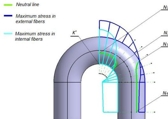
**Figure 6** - Neutral line and the diagrams of maximum stress in internal and external fibers
