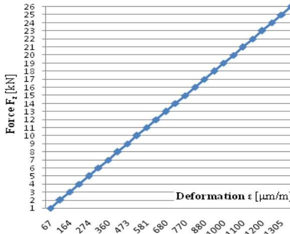
**Figure 15** - Diagram of deformations dependance from the force
