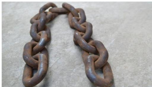
Figure 1 - Appearance of the oval welded long links chain used for the analysis
