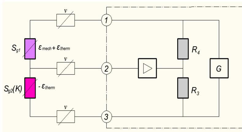
Figure 14 - Electrical scheme of connection of Viston bridge
