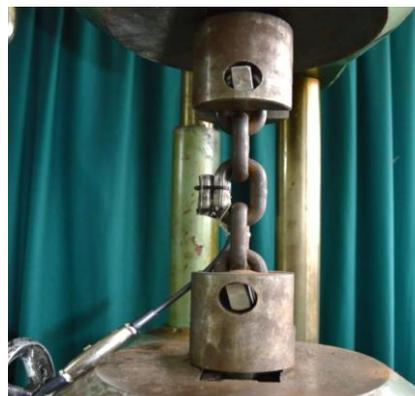
Figure 11 - The chain with strain gauges set in the jaws of testing
