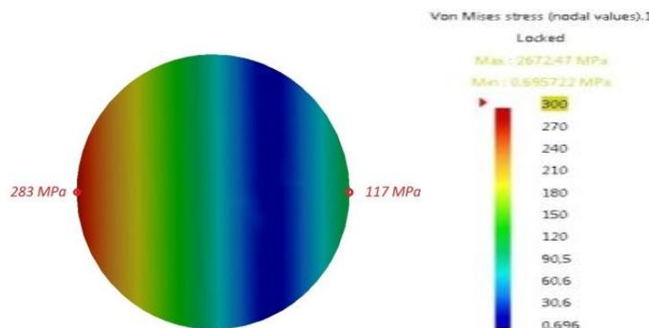
**Figure 8** - The value of Von Mises stress in the middle of the link loaded with 26kN
