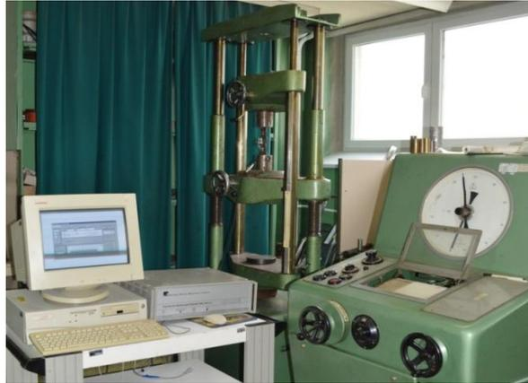
Figure 12 - Equipment for measuring tapes stress analysis
