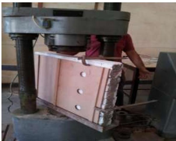
**Figure 11.** Carrying wall on testing machine by wood panels
