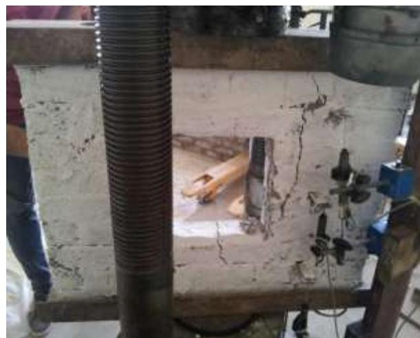
**Figure 2.** Cracks around window opening
