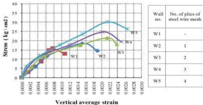
**Figure 14 .** The relationship between stress and strain for control and strengthened walls by using horizontal plies of steel wire mesh embedded into bed joint mortar (one, two three and four plies)
