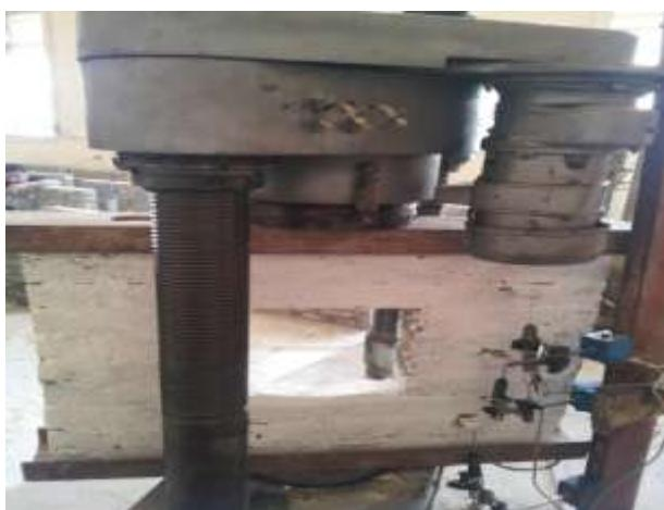
**Figure 13.** Test set up with LVDT
