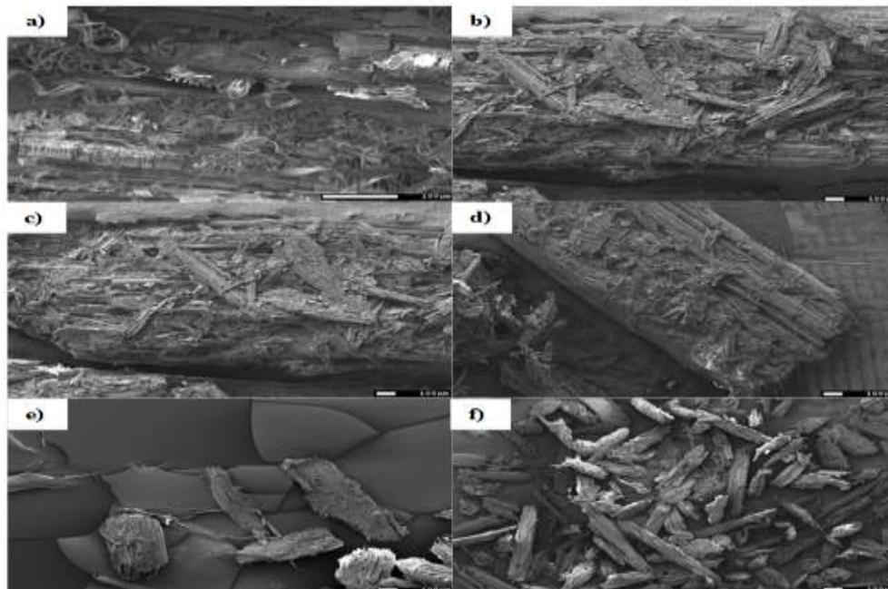
**Fig. 3.** The hemp shives: a) shives slices typical (fractions 2.5÷5.0÷10.0 mm, magnification x200); b) chopped hemp shives (fraction 3.15 – 5.6 mm, x50); c) chopped hemp shives (1.25 – 3.15 mm, x50); d) chopped hemp shives (0.315 – 1.25 mm, x50); e) chopped hemp shives (0.16 – 0.315 mm, x50); f) chopped hemp shives (0.10 – 0.16 mm, x50)
