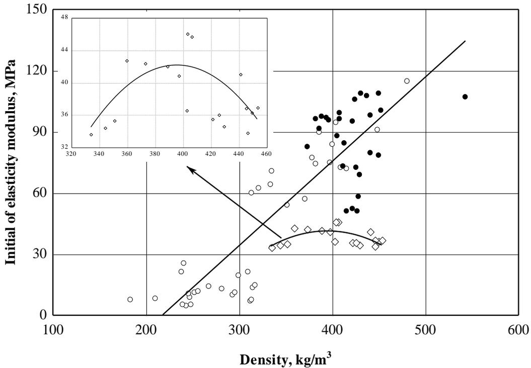
**Fig. 5.** The dependence of initial modulus of elasticity  $\bar{E}$  of hemp shives composite specimens on their density.  $\circ$  – experimental data of hemp shives with starch;  $\bullet$  – experimental data of hemp shives with starch and kaolin;  $\diamond$  – experimental data of chopped hemp shives; — empirical line of regression dependence of specimens' initial modulus of elasticity  $\bar{E}$  on their density
