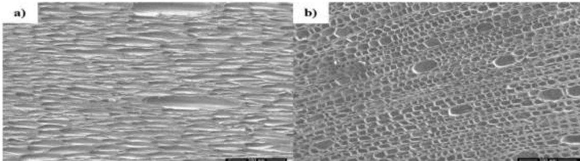
**Fig. 2.** The cellular structures of hemp shives (magnification x200): a) parallel; b) perpendicularly
