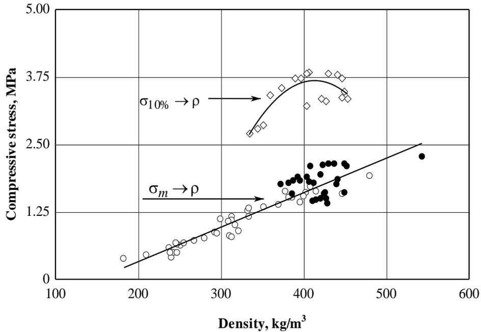
**Fig. 4.** The dependence of ultimate compressive stress  $\bar{\sigma}_m$  and  $\bar{\sigma}_{10\%}$  of hemp shives composite specimens on their density. ○ – experimental data of hemp shives with starch; ● – experimental data of hemp shives with starch and kaolin; ◇ – experimental data of chopped hemp shives — empirical line of regression dependence of specimens' ultimate compressive stress  $\bar{\sigma}_m$  on their density
