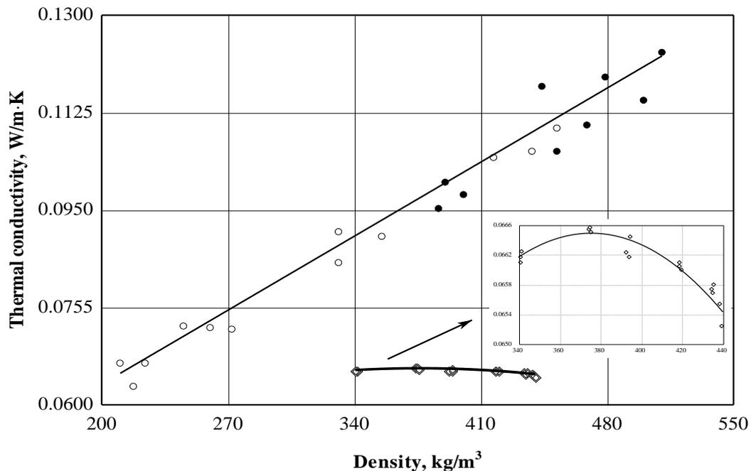
**Fig. 7.** The dependence of thermal conductivity  $\bar{\lambda}_{10^\circ C}$  of hemp shives composite specimens on their density. ○ – experimental data of hemp shives with starch; ● – experimental data of hemp shives with starch and kaolin; ◇ – experimental data of chopped hemp shives; — – empirical line of regression dependence of specimens’
