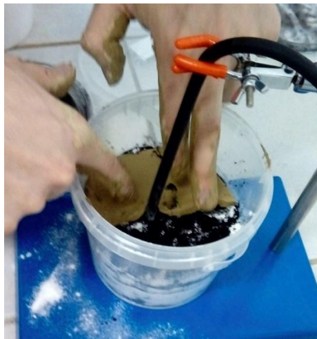
Fig.3. An argillaceous layer follows after the salt with baking soda powder in order to assure a better system
