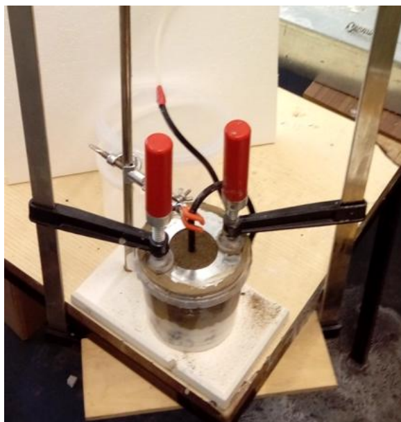
Fig. 1. Vessel prepared with starch and sand under “artificial lithostatic pressure”
