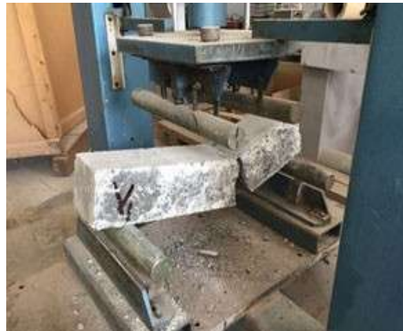
Fig. (15). Failing pattern of steel fibers reinforced concrete under flexural strength test.
