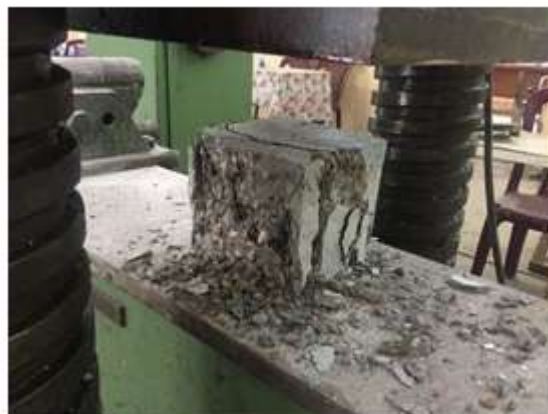
Fig. (11). Failing pattern of SFRC under compression test.
