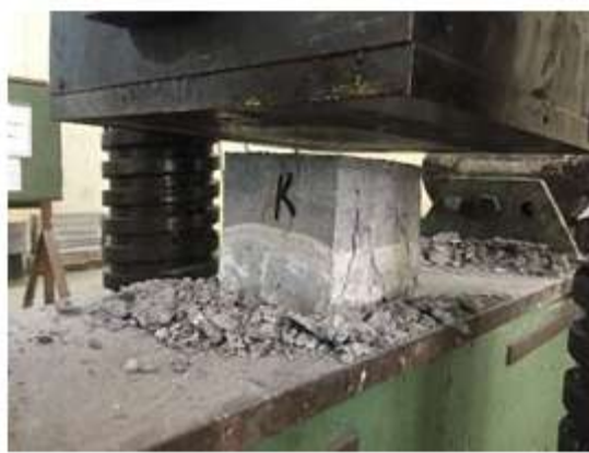
Fig (13). Failing pattern of HFRC under compression test.
