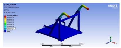
Figure 5. Frame total deformation analysisby ANSYS 15.0
