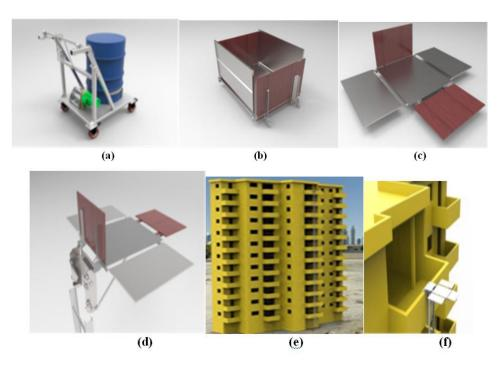
Figure 3. Modeling by SOLID WORK16 (a) Rendering of balcony crane (b) rendering of material holder car closed (c) rendering of material holder open (d) Rendering of material holder guide and support assembly (e) balcony crane fully assembled isometric view (f) balcony crane with condominium building
