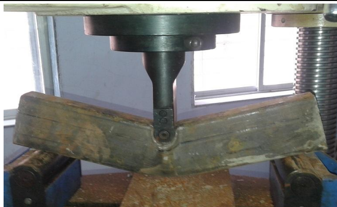
Fig.9 Failure of the composite beam section
