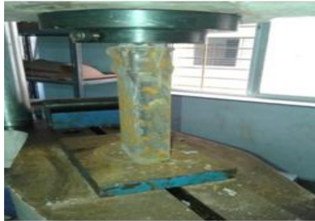
Fig.7 Failure of NFCR-C
