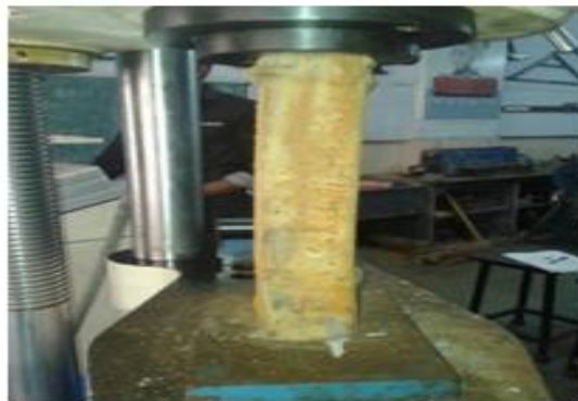
Fig.2 Failure of NMS-C
