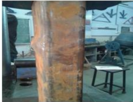
Fig.1 Failure of NCS-C
