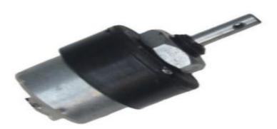
Geared Dc Motors Can Be Defined As A N Extension Of Dc Motors A Geared Dc Motor Has A Gear Assembly Attached To The Motor. The Speed Of Motor Is Counted In Terms Of Rotations Of The Shaft Per Minute And Is Termed As Rpm .The Gear Assembly Helps In Increasing The Torque And Reducing The Speed.
