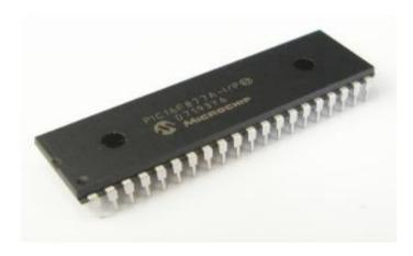
It Is The Heart Core Of The System To Which All Other Components Are Interfaced .Pic Microcontroller Is A Risc Microcontroller Made By Microchip Technology .It Is 40-Pin Low Power ,High Performance Microcontroller .
