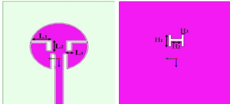
Fig. 2. Geometry of the proposed penta-band antenna
