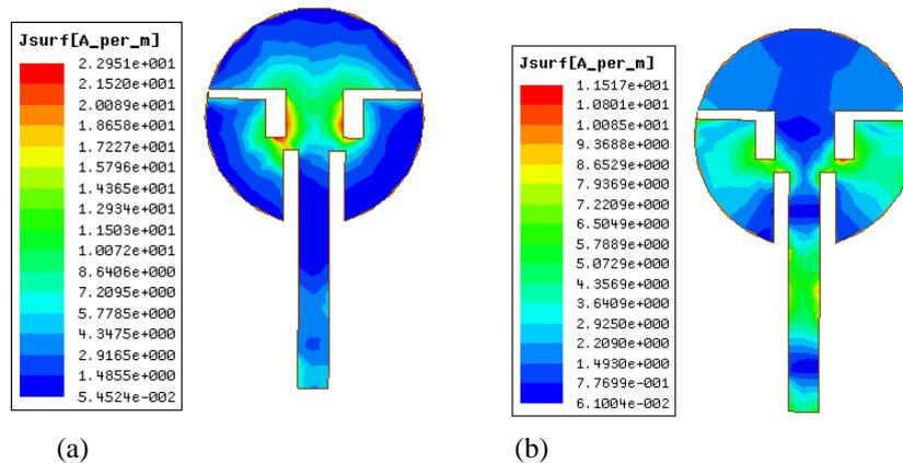
**Fig. 6:** Simulated surface current distributions of the proposed penta-band antenna observed at (a) 2.13 GHz, (b) 5.18 GHz
