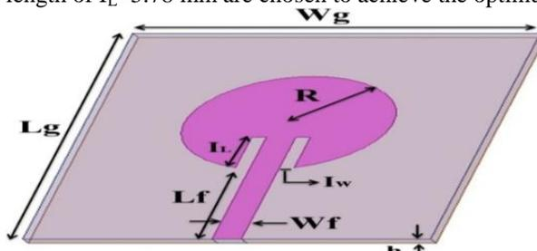
Fig. 1 Geometry of the conventional inset-fed circular microstrip antenna
