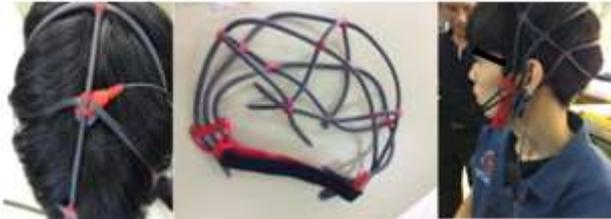
The installation of EEG and MINICAP
