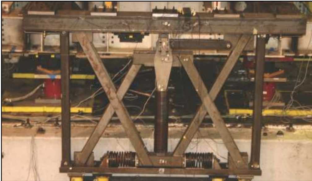
Figure 2.1 A view of Negative Stiffness Damper (Nagarajaiah et al, 2013)
