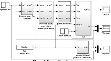
Figure 4. Design Plant System
