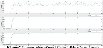
Figure7.Current MotorSpeed Chart 15Hz (Open-Loop)
