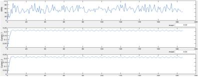
Figure 6.Current MotorSpeed Chart 10Hz (Open-Loop)
