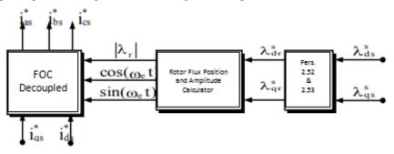
Figure 2. Block Diagram Decoupled Induction Motor
