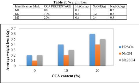
Figure 1: Weight loss of cubes cured in 5% chemical solutions
