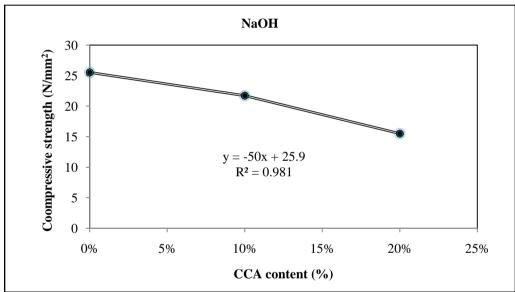
Figure 5: Compressive strength of CCA concrete cured for 90 days in 5% sodium hydroxide solution
