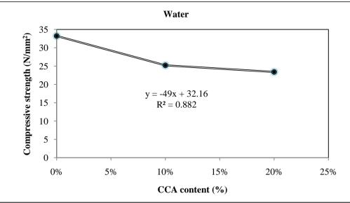
Figure 7: Compressive strength of CCA concrete cured for 90 days in water
