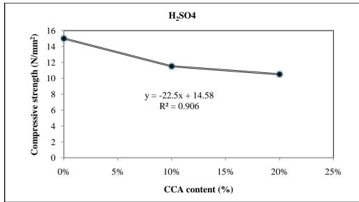
Figure 4: Compressive strength of CCA concrete cured for 90 days in 5% sulphuric acid solution
