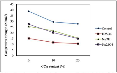
Figure 3: Comparison of compressive strength of concrete cured for 90 days in 5% chemical solutions
