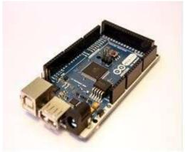
figure 3 Arduino micro-controller
