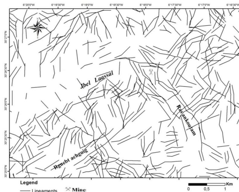
Figure 4: Synthetic map of lineaments extraction from Sentinel-2A image
