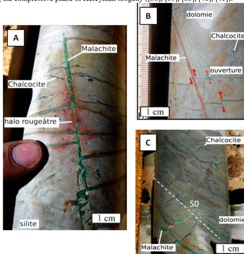
Figure 12: Photograph of drill core: A; Malachite-fill connected fractures, B; Malachite-fill fractures offset by a second reverse set fracture, C; mineralization in the form of Stockwork parallel and oblique to the stratification.
