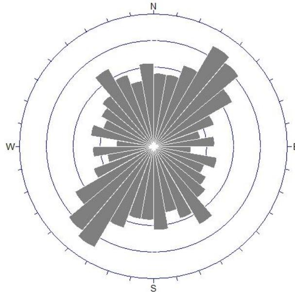
Figure 5 : Rose diagram of lineaments extract from Sentinel-2A image
