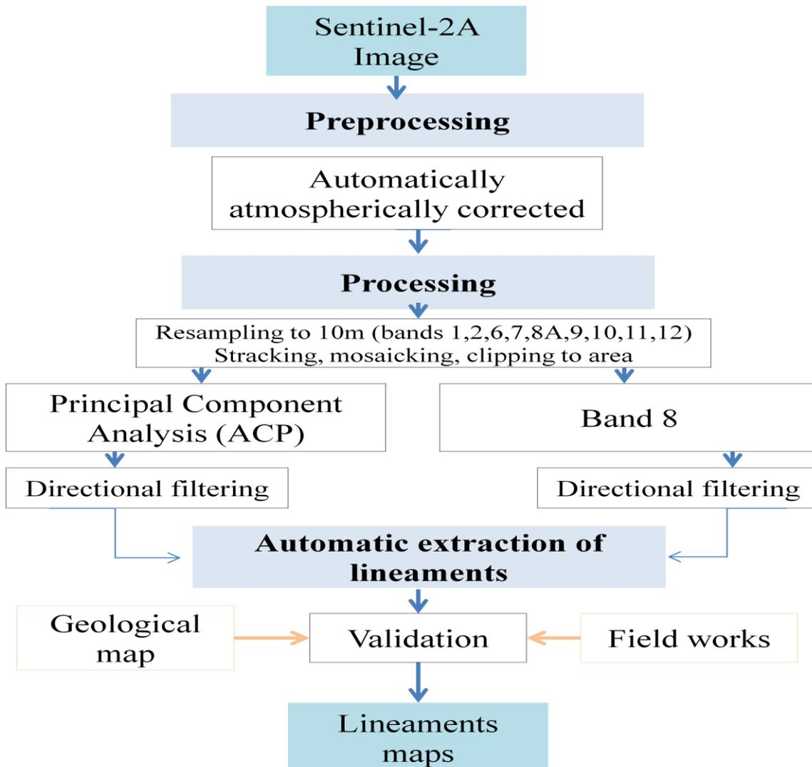
Figure 2: Methodology flowchart used in this study of lineaments extraction
