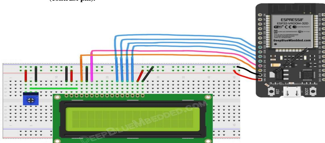
Fig Interfacing LCD module with ESP32 Microcontroller
