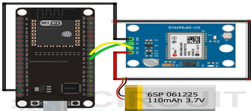
Fig Interfacing GPS module with ESP32 Microcontroller
