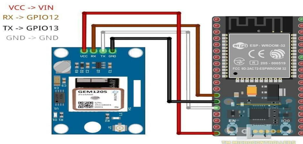
**Fig** Interfacing GSM module with ESP32 Microcontroller
