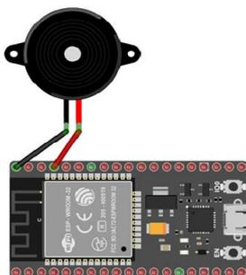
Fig Interfacing Buzzer with ESP32 Microcontroller
