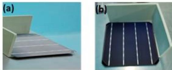
Fig.10. The image of monocrystalline Si solar cells (a) without SiN<sub>x</sub> film (b) with SiN<sub>x</sub> film.
