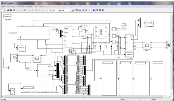
Fig 5 Designed model that reduces power losses in transmission network using optimization
