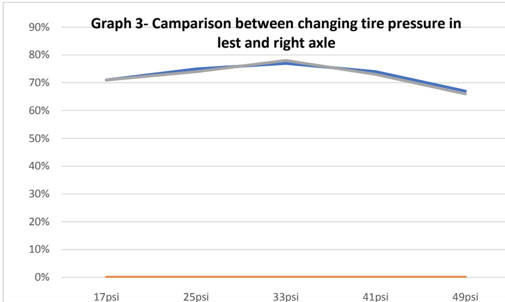
The graph shows changing of the inside tire has a similar effect on road grip of left and right axle.
