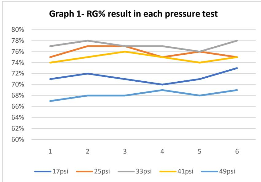
The graph 1 shows while the road grip is maximum level in nominal pressure which is suggested by car manufacturer, both decreasing or increasing of pressure by 8 psi will deduct road gear percentage proportionally from 2% to 4%
