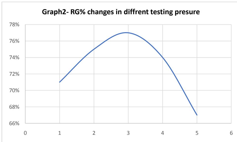
Graph 2 shows the relation between changing the inside pressure with changing of road grip is an exponential function. While inflation of tire has more effect on decreasing the road grip than being under pressure.
