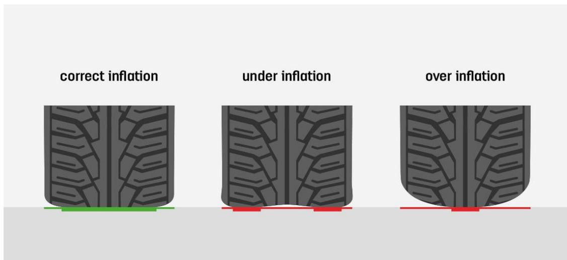
In the case of inflation, the tire profile, which is consistent with the above-mentioned data, reveals less tire contact with the earth, resulting in reduced road grip and braking force.
