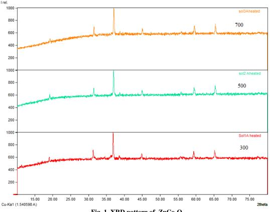
Fig. 1. XRD pattern of ZnCo<sub>2</sub>O<sub>4</sub>.
