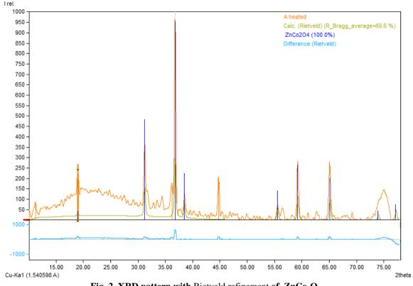
Fig. 2. XRD pattern with Rietveld refinement of ZnCo<sub>2</sub>O<sub>4</sub>.
