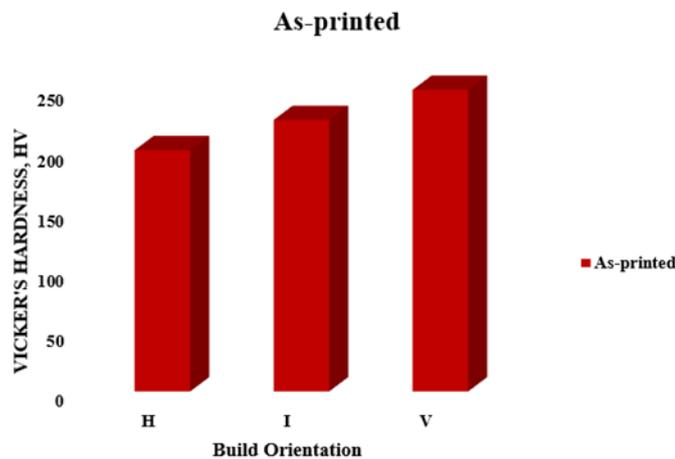
**Figure 8: Effect of build orientation on as-printed(non-heat-treated) 17-4-PH SS**
