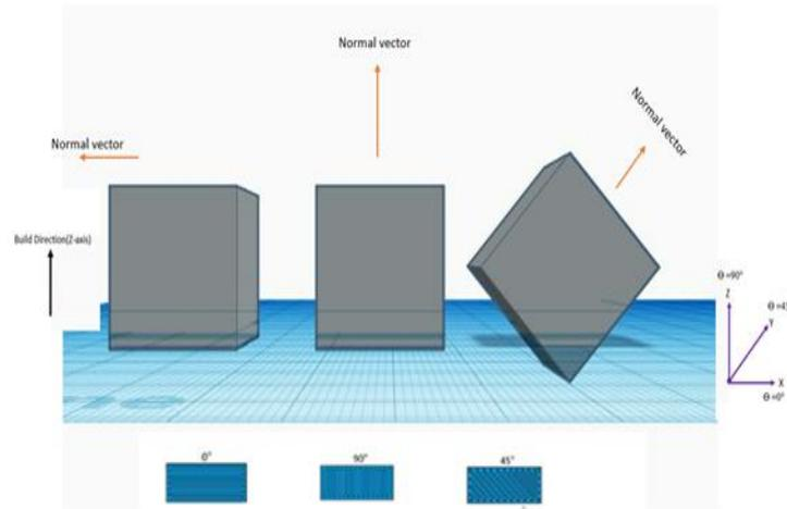
**Figure 1 shows three build orientations of the samples.**
