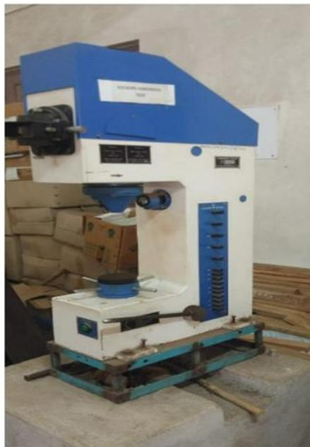
**Figure 3 shows Vicker's hardness tester**
