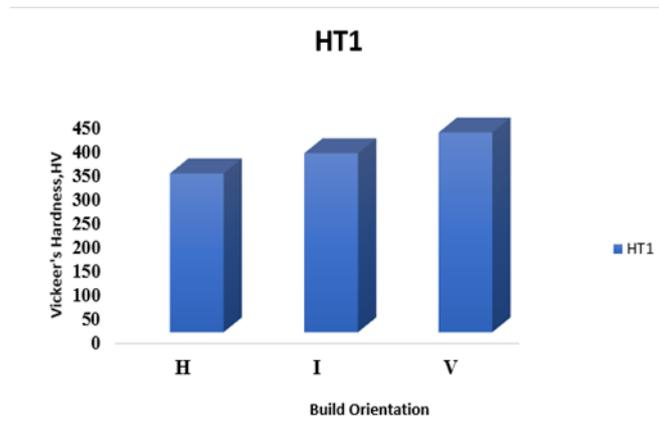
**Figure 4: Effect of HT1 on hardness and orientation of 17-4-PH SS**
