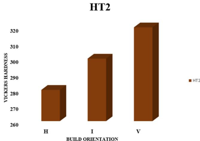
**Figure 5: Effect of HT2 on hardness and orientation of 17-4-PH SS**
