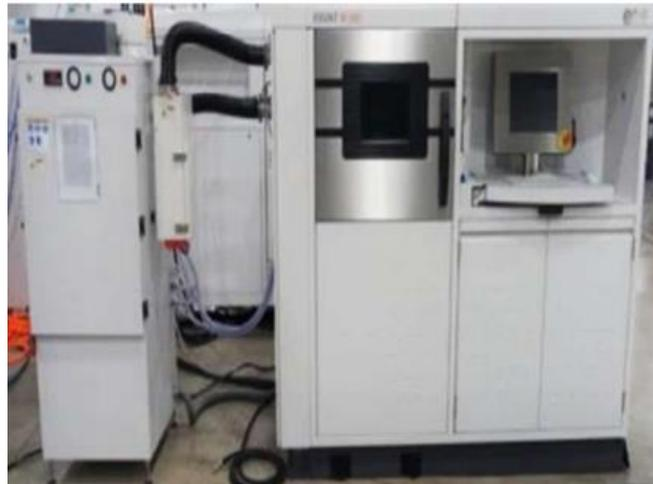
**Figure 2 shows Laser powder bed fusion system EOS M-290**
