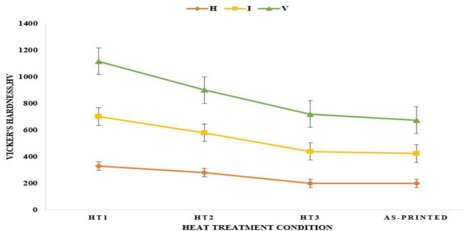
**Figure 7: Effect of various Heat treatments on hardness and orientation of 17-4-PH SS**
