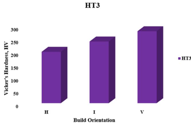
**Figure 6: Effect of HT3 on hardness and orientation of 17-4-PH SS**
