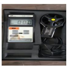
**Plate 5 Anemometer**
