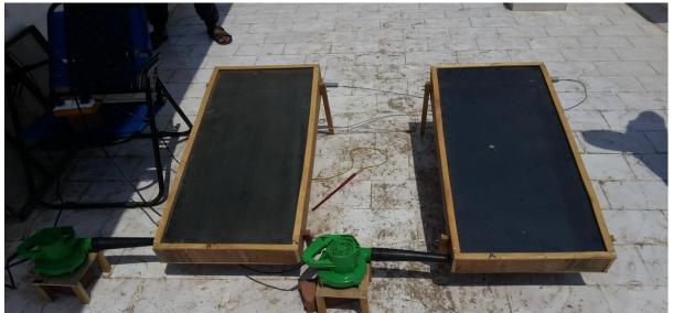
Plate 6 Experimental Set up of Conventional and V trough Solar Air Heater
