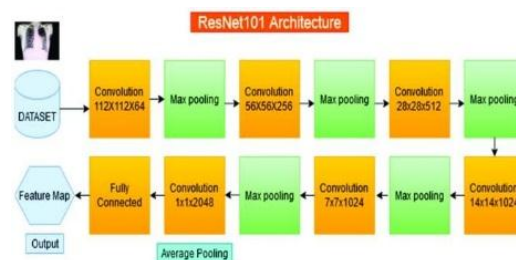
Fig.1. Architecture of Resnet101
