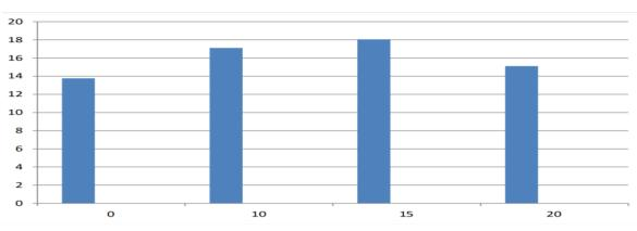
NOTE : ON X – AXIS PERCENTAGE OF PHOSPHOGYPSUM (%) ON Y – AXIS COMPRESSIVE STRENGTH (N/mm2 )
