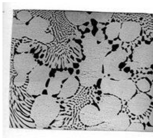
Figure 7: As cast structure (SEM) of Alloy No3 at medium magnification(350x) showing former \beta attached to primary \eta dendrites
