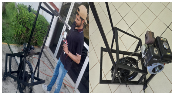
Figure 5. Finished prototype of the furrower. Source: Own elaboration.
