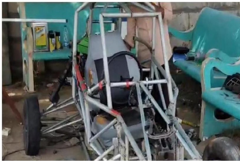
Fig. 1: Fabricated cross-kart with the twin-charged single-cylinder engine
