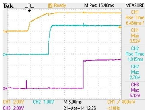
Fig. 3 – Power On Reset Generation & Power Sequencing
