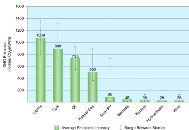
**Fig 3:** Lifecycle GHG Emissions Intensity of Electricity Generation Methods (World Nuclear Association, 2011).
