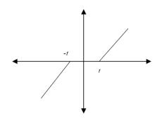
Figure 12: Soft thresholding
