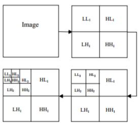
Fig. 10: 3 level discrete wavelet decomposition
