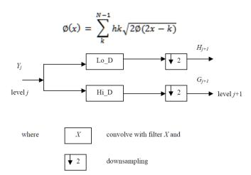
Fig. 9: A 1-Dimensional DWT - Decomposition step
