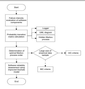
Fig. 1. Schema of method for software reliability analysis based on HOMC.
